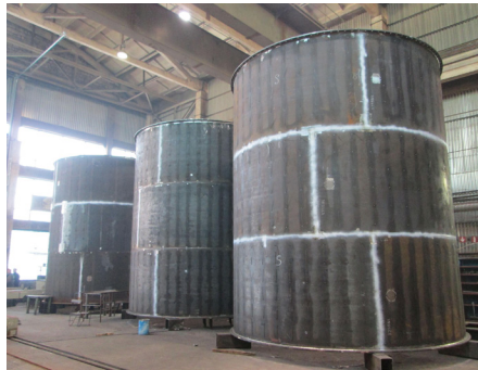
Liner manufacturing and storage before implementation
