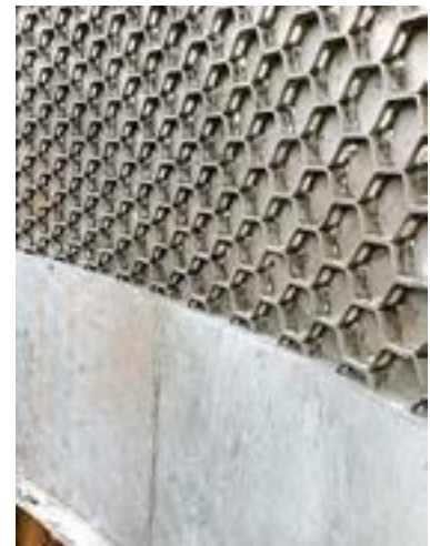
Hex-mesh for AA22 Rescobond material & Rescicast 17EC
