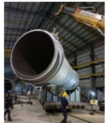
Segment relocation for lining installation
