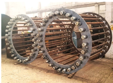
Anchorage ring fabrication
